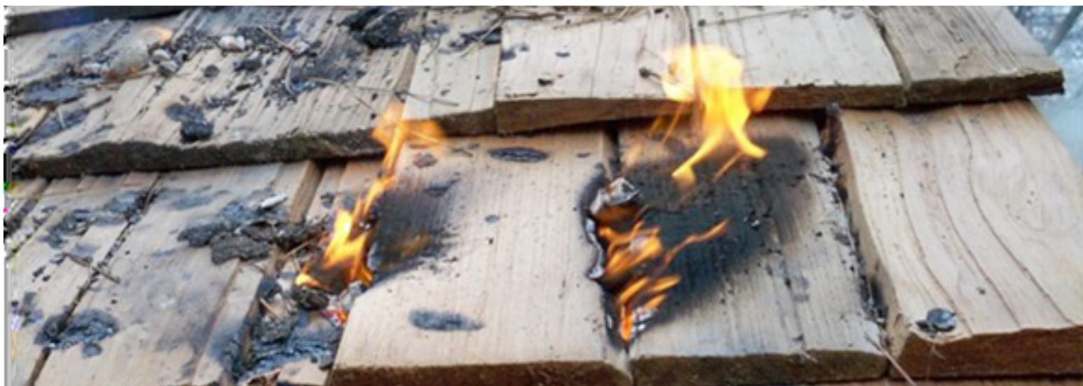
Wood shake shingles can easily ignite when firebrands are caught in their crevices Photo by David Yegge
